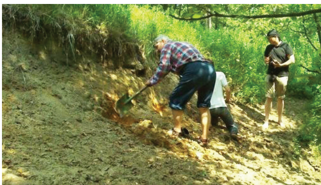
Fig. 2, 3: Mining bog iron ore which situated in bog iron ores form lenses close to the surface of the ground. These lenses can be found in the beds of brooks, where the brook has eroded one to two metres below ground level
