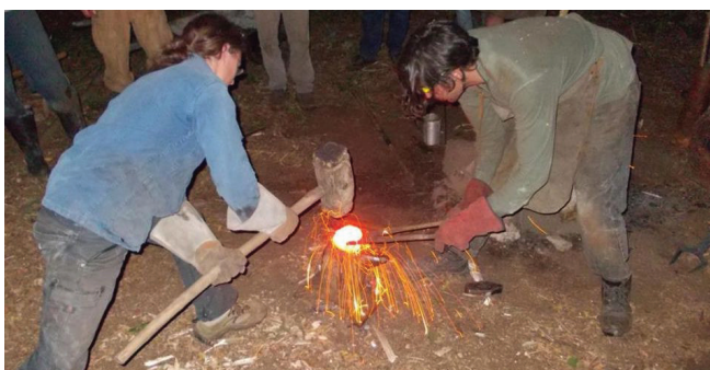
Fig. 5: Forging the iron bloom to bar
