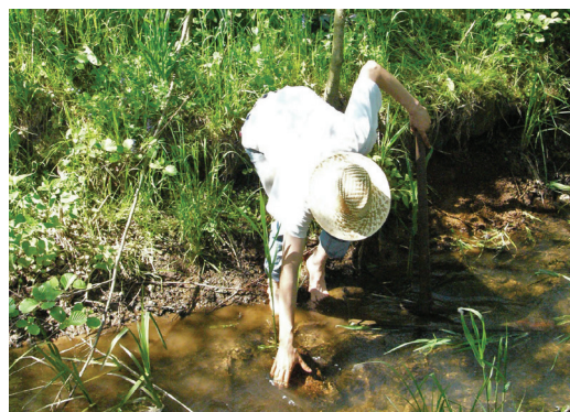
Fig. 2, 3: Mining bog iron ore which situated in bog iron ores form lenses close to the surface of the ground. These lenses can be found in the beds of brooks, where the brook has eroded one to two metres below ground level
