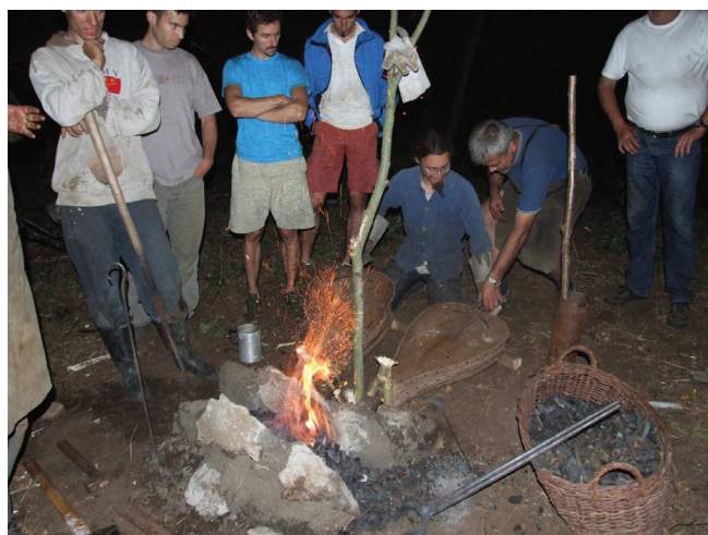
Fig. 6: Forging the iron bloom to bar
