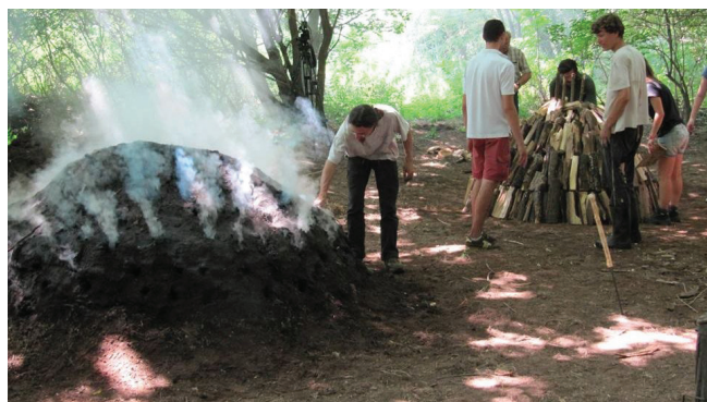
Fig. 5: Burning charcoal in two charcoal piles of 1–2 m 3 volume. The place of the camp is in a forest near to a brook where a ca. 300m 2 free area is provided for the participants
