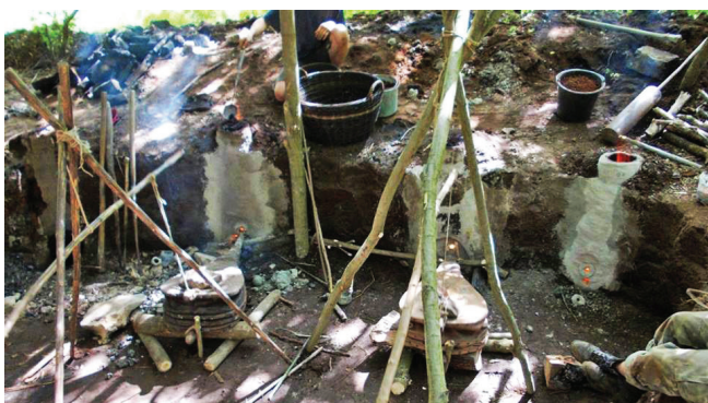
Fig. 4: Iron smelting in reconstructed bloomery furnaces
